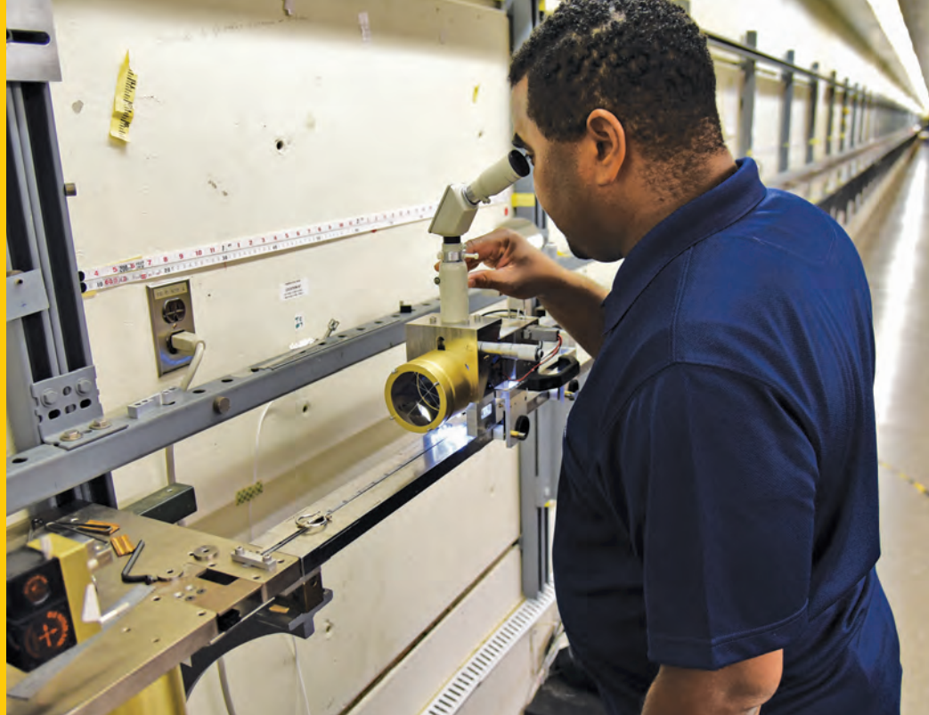
Sawyer calibrates tapes by looking at their graduations or hash marks through a microscope. Credit: F. Webber/NIST
