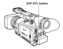
Press EVF DTL again to return to the original display. "EVF DTL OFF" appears on the screen for about 2 seconds.
