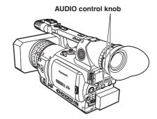
Use the AUDIO control knob to adjust the recording level of the built-in microphone or of audio signals input through the INPUT 1/2 (XLR 3-pin) terminal.
