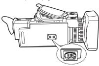
Attach the tripod to the tripod hole.
