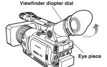
Do not point the eye piece at the sun. Doing so may damage the parts inside. Fitting the eye cup
