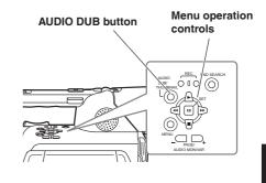
Audio dubbing cannot be performed in the LP mode because the track width on the tape is narrower than the head width.
