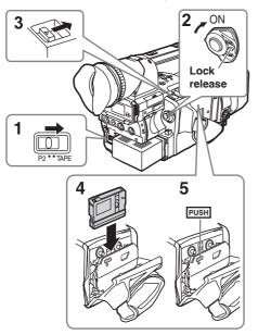
Do not operate the MEDIA switch when the power is switched ON.
