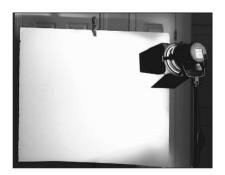
ARRILITE BOUNCING OFF OF FOAM CORE BOARD
