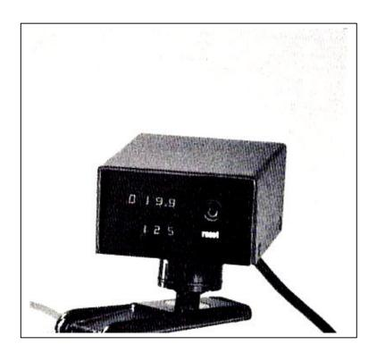
separated from its battery. The EFC-16 SR can be connected directly via a cable with the camera's electronic shoe. (Socket 45); when the VSU is used with the EFC-16 SR, the accessory distributor ZV is necessary. The counter is attached to the additional thread (40) on the camera carrying handle; the ball and socket joint connection enables the EFC-16 SR to be positioned in any direction !or easy reading.
