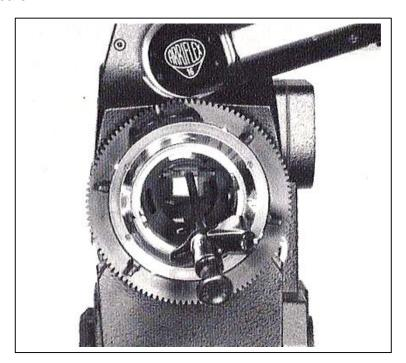
Should it be necessary to remove the fibre optic viewing screen this operation is carried out with a special clamp inserted in the lens bore. Care must be taken when reinserting the fibre optic viewing screen that it is securely seated, otherwise the image reproduced on the film and the image seen in the viewfinder will not be identical.
