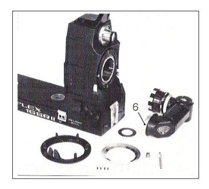
and the primary optics must also be removed. The video adaptation is mounted reversing the above-described steps. The friction disc is not used. Care must be taken that the adapter arm for securing the viewfinder (seen in taking direction) is on the left side of the camera housing. It is not possible to turn the video adapt ion through 180° for left eye viewing.
