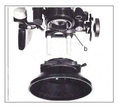
The light-weight support is placed in the camera shoe (19) and fastened with the knurled screw (a) which is found between the two support rods. The accessories can now be pushed on the rods, positioned as required, and held secure by tightening the screw (b).
