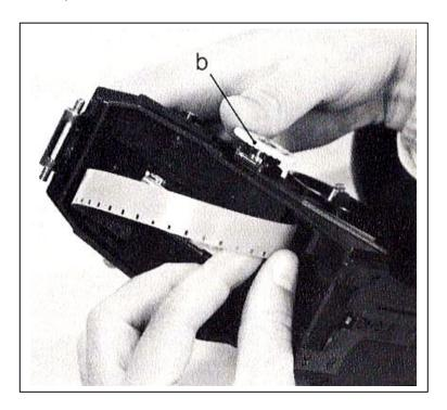
When a plastic film core is used, the standard film holder is pushed onto the wind-up pole until it engages and the plastic film core is then pushed onto it. The slit for fastening the film must point with its pointed corner in the run direction. The film-head should only be folded *once* (NOT several times) and inserted into the film core slit; the film is then made taut as described above.
