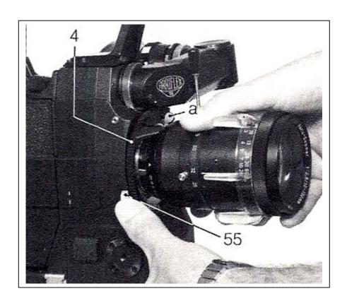
To mount lenses with steel bayonet mount: the diaphragm lever (a) is inserted into the slot of the catch ring (4), the lens (white index mark positioned as stated above) is carefully pushed into the lens mounting flange and turned clockwise until it locks.
