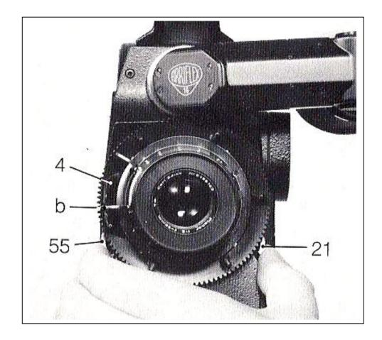
To mount lenses with standard mount: the diaphragm lever(b) is inserted into the slot of the catch ring (4). Both buttons (21, 55) are simultaneously pressed and held together and the lens (index mark positioned towards the exposure meter) is carefully pushed into the lens mounting flange. The catch in the lens mount then engages in the guide groove of the lens barrel. Release the buttons and check that the lens is firmly seated. -
