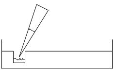
Figure 3. Correct position of tip when filling well.
