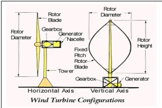
Figure 1 Horizontal-axis turbines are comprised of a rotor or blades, drive train, generator, tower, and electronic equipment (AWEA 2004a).
