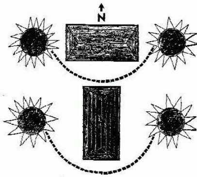
Figure 6.1. East-west orientation of the home. With the long axis built as above, the smaller sides of the home receive less hot summer sun than the long walls would if oriented differently.
