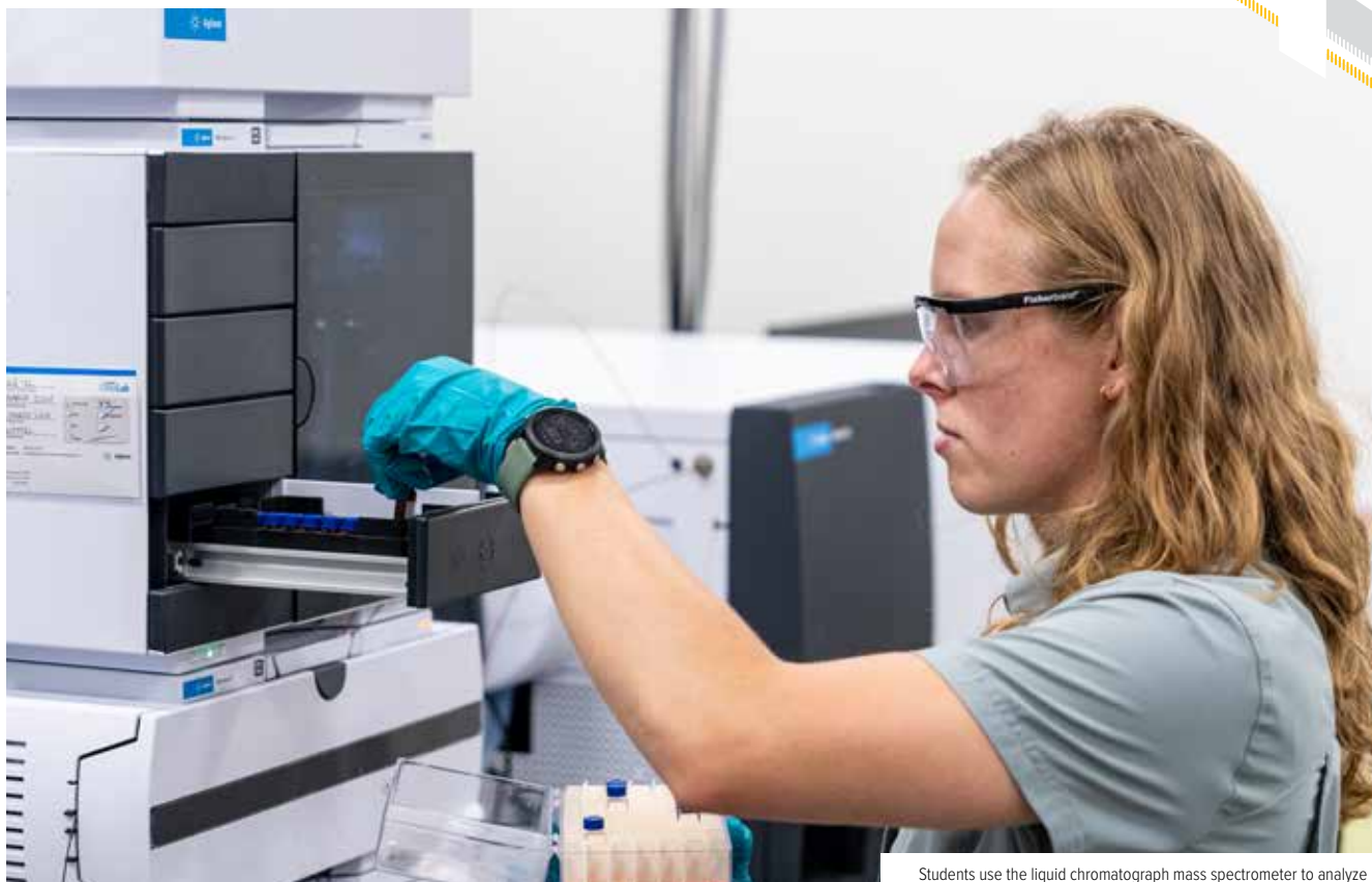
Students use the liquid chromatograph mass spectrometer to analyze samples, using both parts of the instrument during the analysis.
