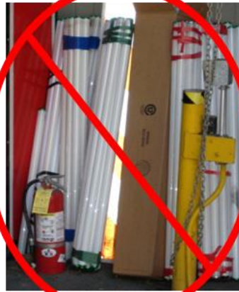
Figure 2. Improper Storage. Bundled lamps stored loosely, leaning upright or slanted against walls with incompatible equipment, risks breakage and penalties.
